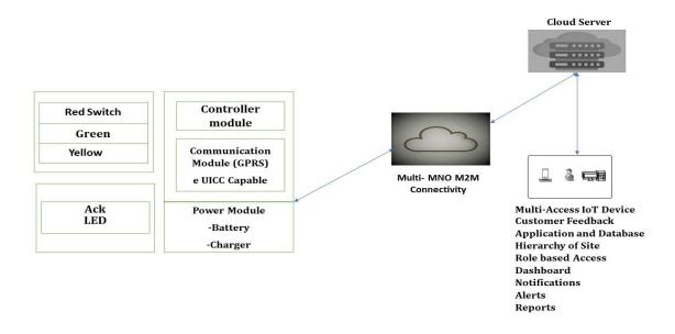
Fig.1 Feedback device architecture
